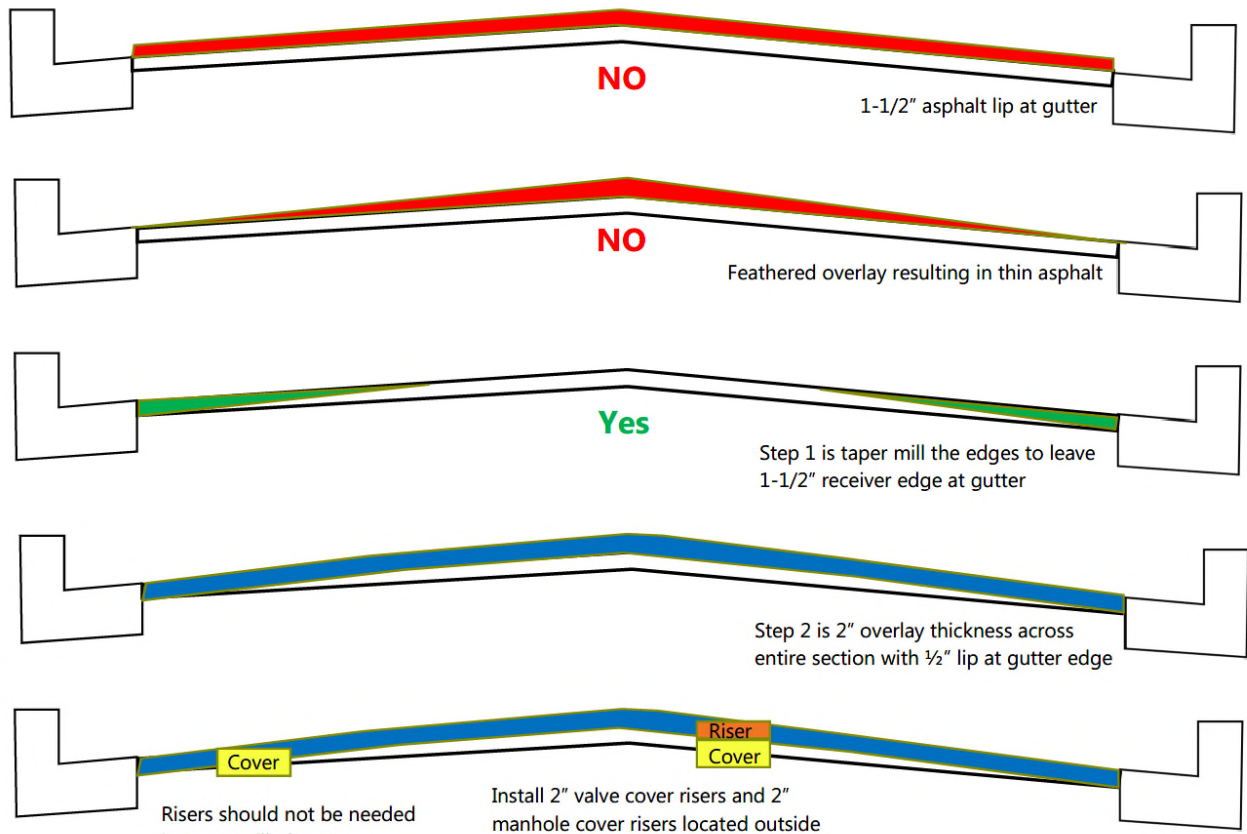
Figure 1: Milling/Overlay Detail
